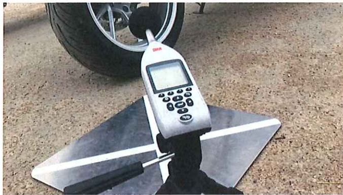
A device used to measure decibel levels on motorcycles can be seen collecting a sample from a Saskatoon police motorcycle in a photo posted to the official Twitter account of the traffic unit with the Saskatoon Police
