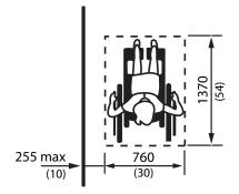
Figure 4.1.1.13 Side Reach - Maximum Distance to Wheelchair
