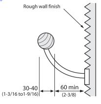
Figure 4.1.12.2 Handrail at Rough Wall
