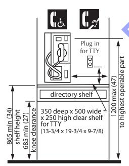
Figure 4.4.5.1 Accessible Telephone
