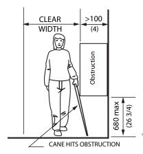
Figure 4.1.3.1 Limits of Protruding Objects
