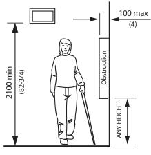
Figure 4.1.3.2 Limits of Protruding Objects
