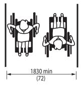
Figure 4.1.4.2 Access Widths
