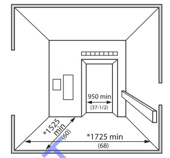
Figure 4.1.14.1 Elevator Cab
