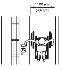
Figure 4.5.4.2 Aisle Width
