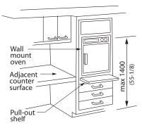
Figure 4.3.18.8 Wall-Mounted Oven
