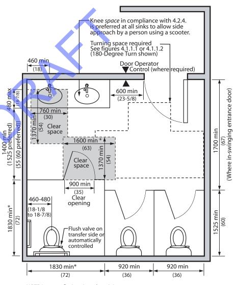
NOTE: In a retrofit situation where it is *technically infeasible* to provide the required clearances, the dimension marked with an \* may be reduced to 1525 mm (60 in.).
