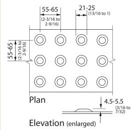
Figure 4.4.8.2 <u>Truncated Dome</u> <u>Detectable Warning Surface</u>
