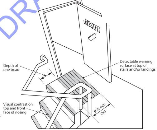
Figure 4.4.8.1 Detectable Warning Surfaces at Stairs
