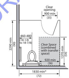
Note: In a retrofit situation where it is *technically infeasible* to provide the required clearances, the dimension marked with an \* may be reduced to 1525 mm (60 in.) and the *clear* transfer *space* may be reduced to 760 mm (30 in.).
