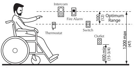
Figure 4.4.2.1 Reach Range for Accessible Controls
