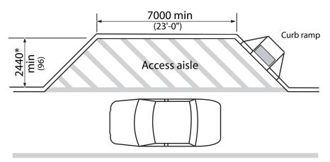
Figure 4.3.13.2 Passenger Loading Zone
