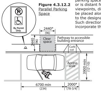
\* NOTE: In a retrofit situation where it is *technically infeasible* to provide the required *access aisle* width, the aisle width may be reduced to 1220 mm (48 in.).
