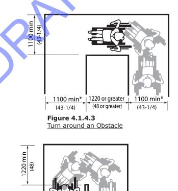
Figures 4.1.4.3 and 4.1.4.4 illustrate interior routes. Dimensions marked \* to be increased to 1220 mm (48 in.) at exterior routes.
