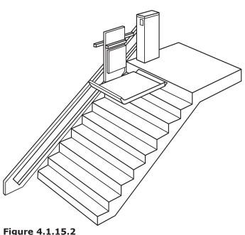
Inclined Platform Stair-Lift
