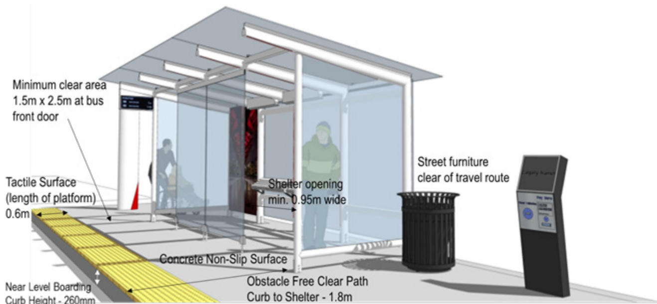
Figure 6. Examples of Station Pad Accessibility Features
