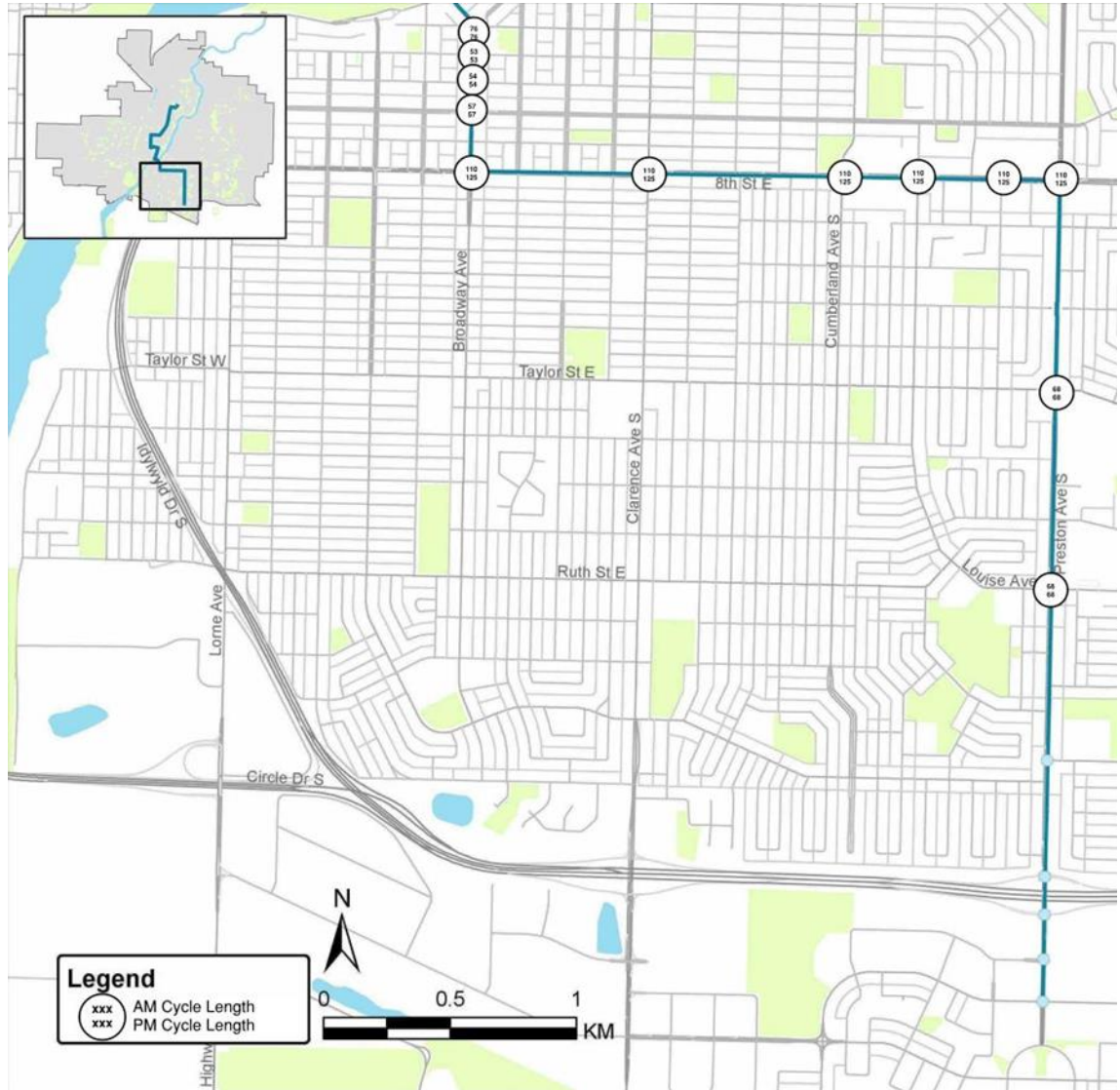
Figure 8-2: Existing Traffic Signal Cycle Length, AM & PM Peak Hour – Blue Line BRT South
