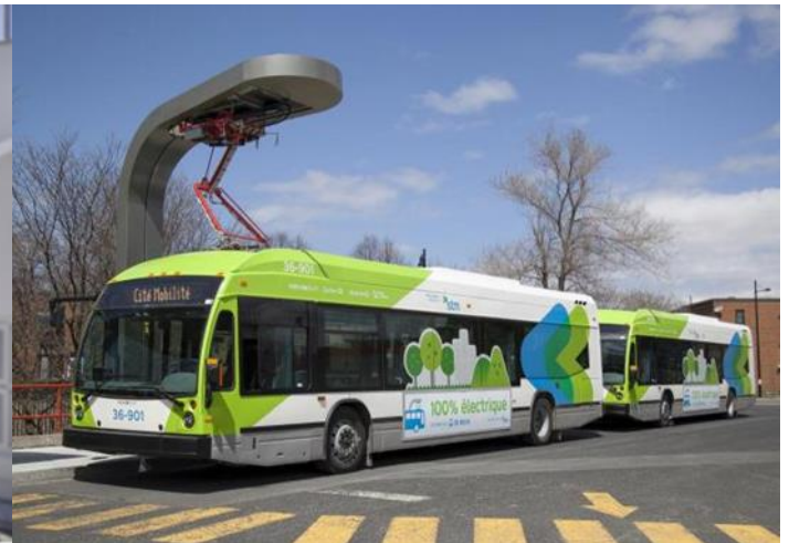
Figure 13: Electric Buses in Montreal at their top-down pantograph charging stations 1
