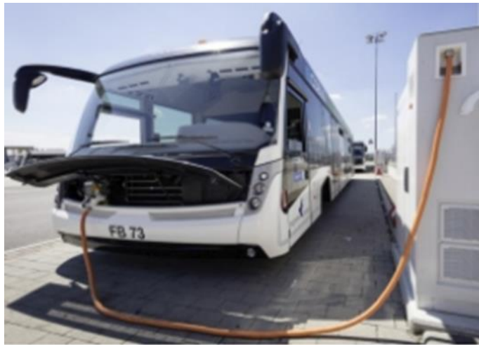
Figure 12: Fast Charging Station using plug-in DC charger
