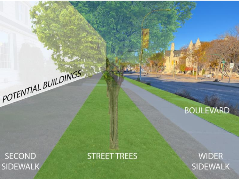
Figure 2: The preferred sidewalk option where there is limited public space, such as along the south side of College Drive, was having trees and a second sidewalk further away from traffic.
