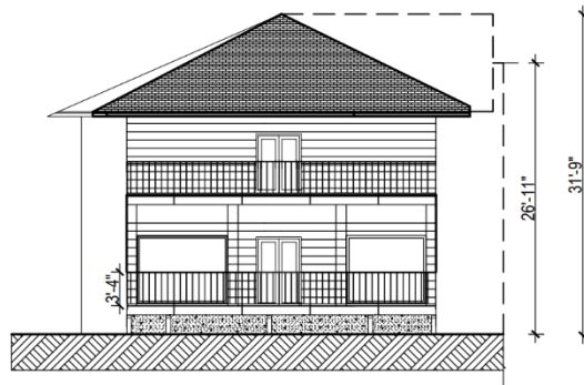
1 | E3 BACK ELEVATION SCALE 3/32" = 1'-0"
