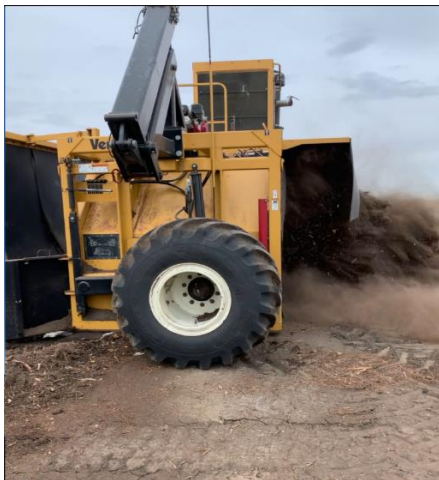
Figure 1 City Owned Compost Turner Aerates and Recombines Composting Materials
