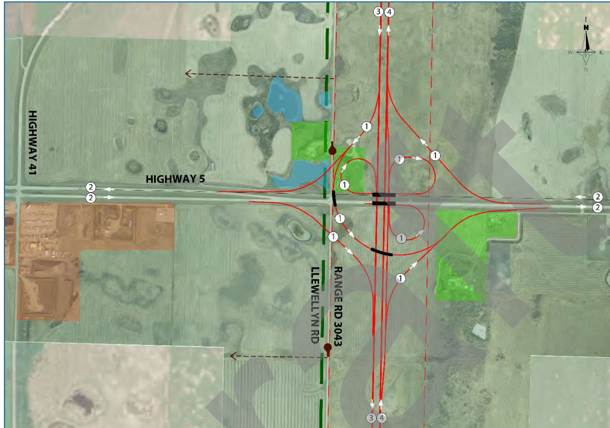
Figure 5.16: Highway 5 Interchange Concept 2
