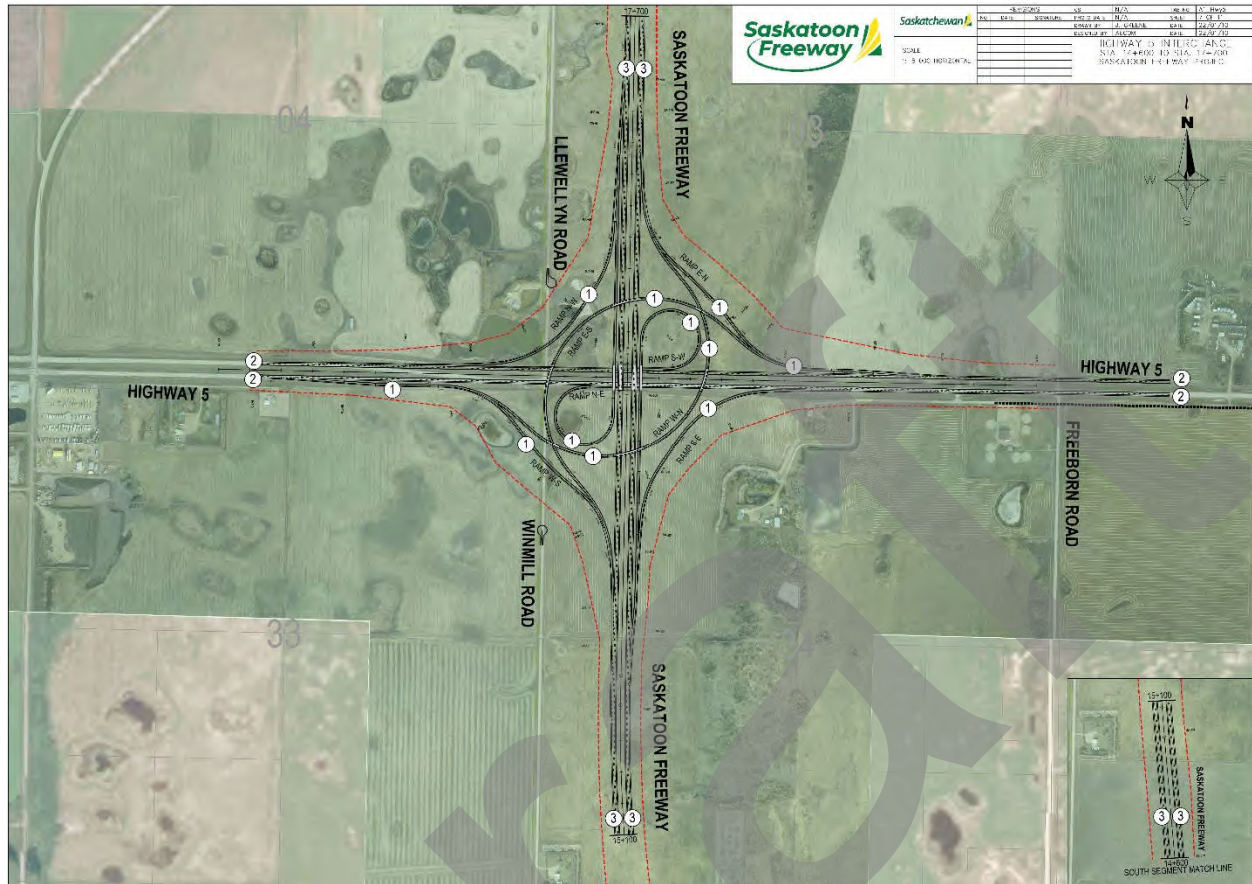
Figure 9.5: Highway 5 recommended interchange configuration
