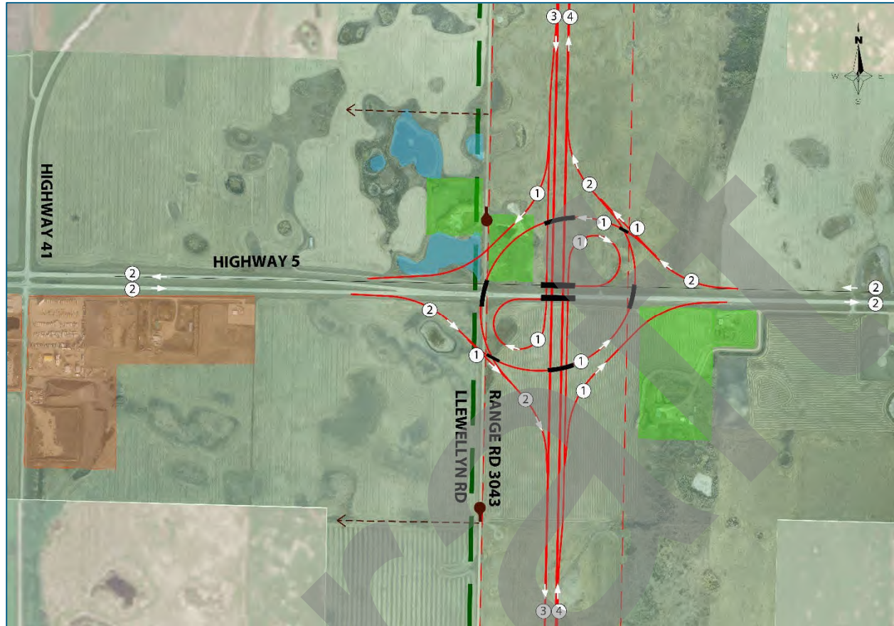
Figure 5.15: Highway 5 Interchange Concept 1
