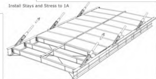
Install Stays and Stress to 1A
