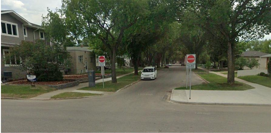
**Figure 2.7: Traffic Diverter on Avenue C at 38<sup>th</sup> Street (Facing South)**
