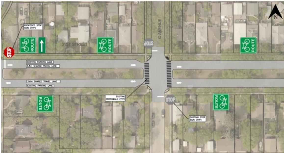
**Figure 2.10: Bicycle Boulevard Conceptual Design for 31<sup>st</sup> Street at Avenue C (Neighbourhood Bikeways Project: 31<sup>st</sup> Street West Corridor, 2020)**
