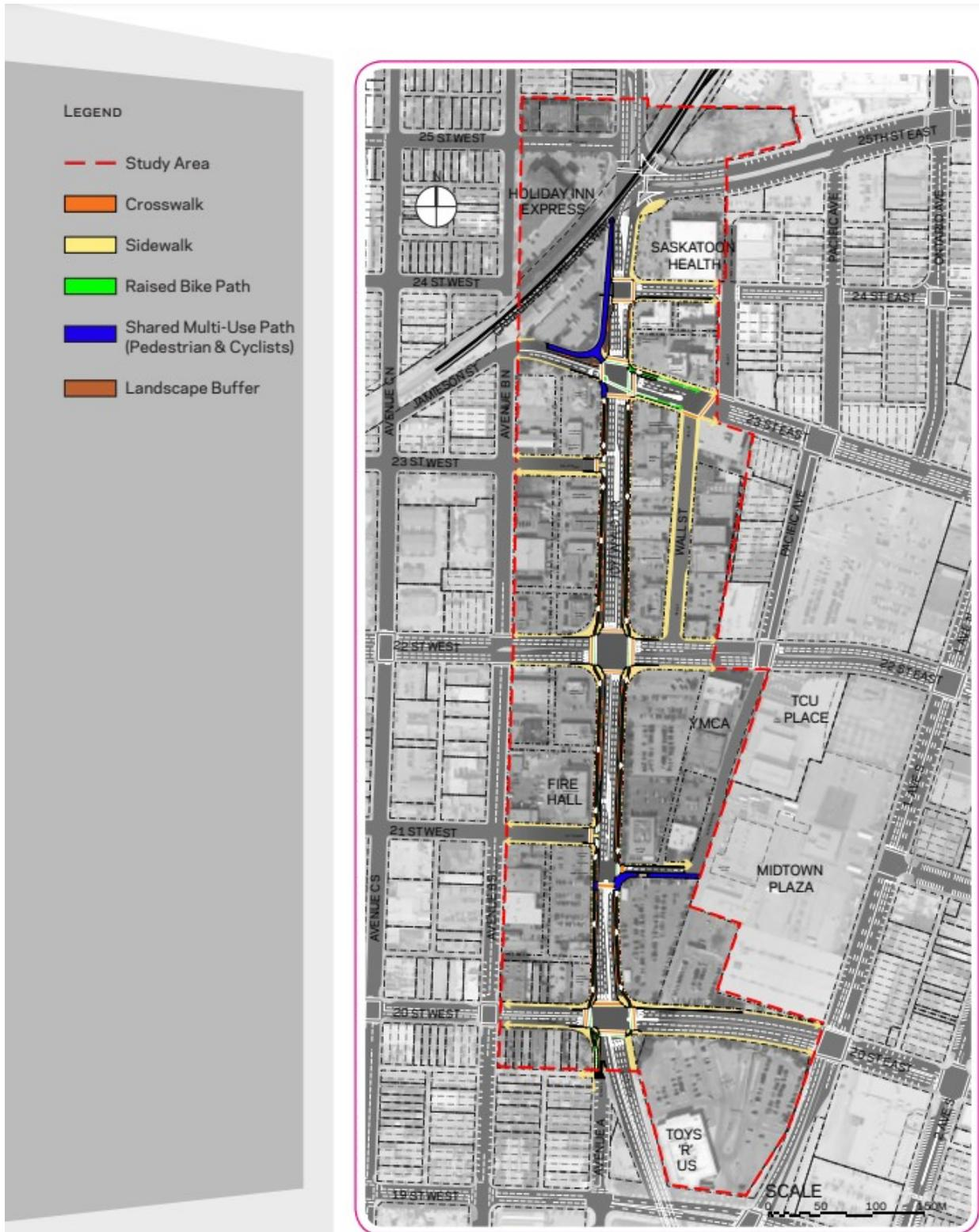
Figure 2.11: Imagine Idylwyld Conceptual Design (Imagine Idylwyld: Conceptual Design Report, 2018)
