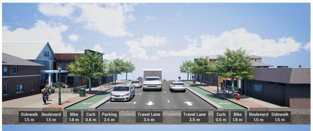
Sample cross section of unidirectional bike lanes on Avenue C.
