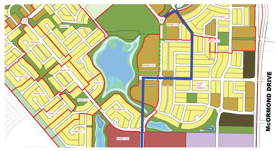
WORK DURING THIS STAGE - Removal of old McOrmond Dr. between 'C' St. and the roundabout, grading of the Phase 11-1 north parcel, and underground and roadway construction along BrightonBlvd. between the roundabout and Tufts Way.
