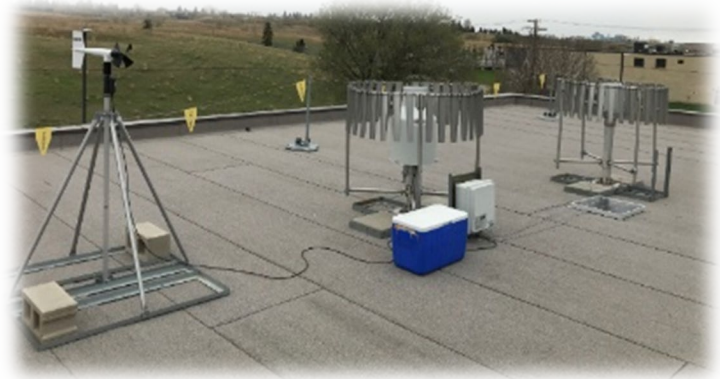
Figure 40: Photograph of Rainfall and Wind Measurement Equipment
