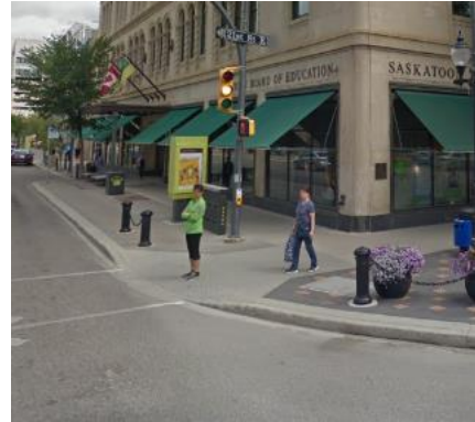
Image 17: Curb Extension Source: Google, Image Capture July 2018
