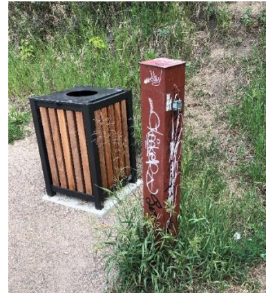
Fig. 4 Well with metal casing and lock
