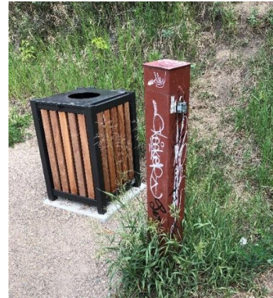
Fig. 4 Well with metal casing and lock
