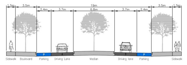
Figure 3: Victoria Avenue - Existing Cross-Section between 7th Street East and 6th Street East
