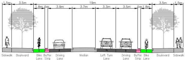
Figure 14: Victoria Avenue - Option 4 - Protected Street-Level Bike Lanes with Parking (8<sup>th</sup> Street East to 7<sup>th</sup> Street East)
