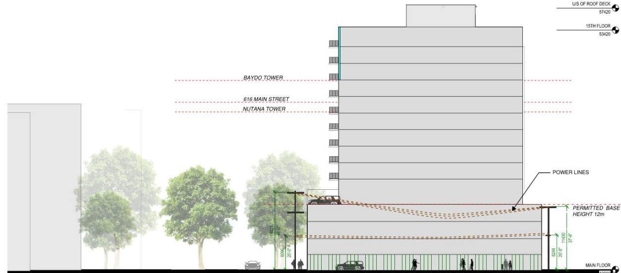
Figure 7. Permitted Buildable Volume, Dufferin Ave Elevation
