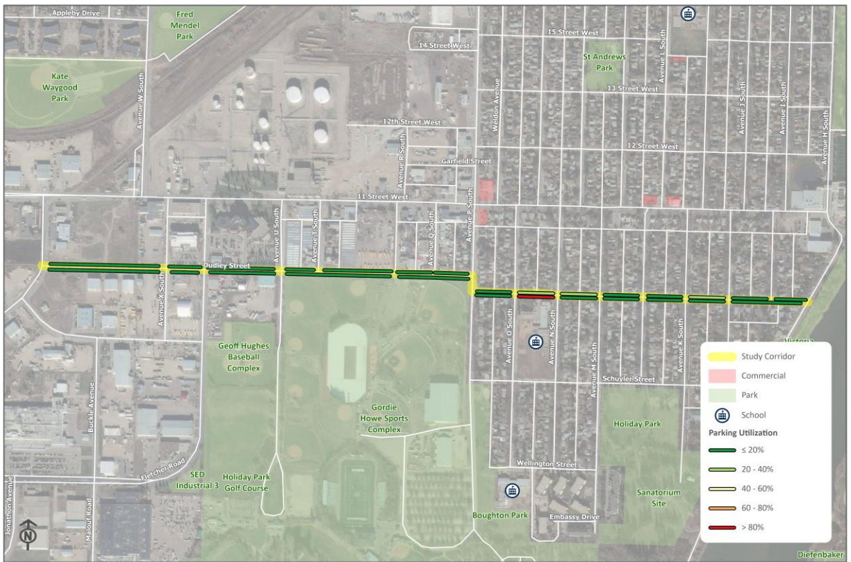
Figure 6. Dudley Street: Mid-day Parking Utilization
