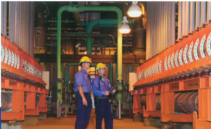
ELECTROLYZER ROOM. Sodium chlorate is produced by the electrolysis of concentrated brine solution.
