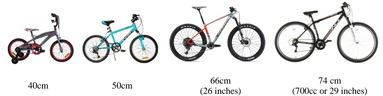
Figure 3- Comparison of wheel diameters
